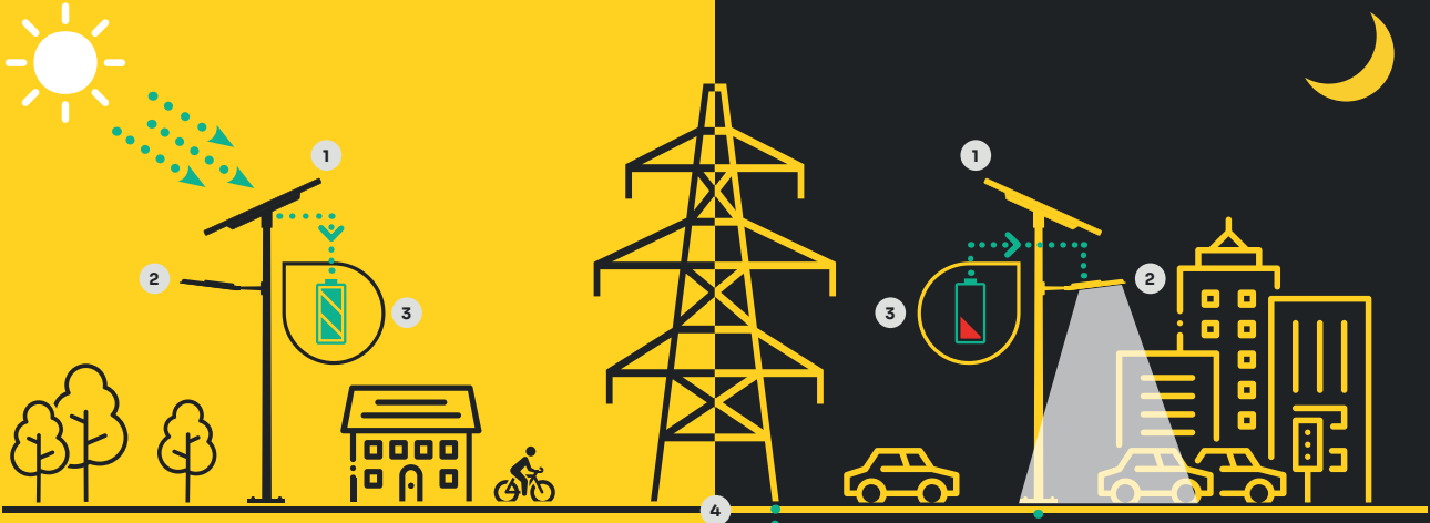
1 Solar panel 2 Fixture 3 Battery 4 Electrical grid
